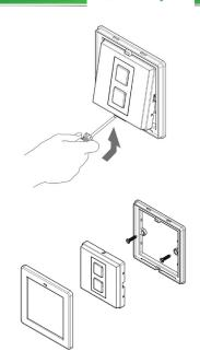
**4.** Replace the centre switch unit and clip the faceplate back into place. Make sure that the faceplate hooks in from the top as shown. A sharp click will indicate that the plate has been successfully replaced.
