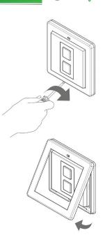
**2.** Insert the screwdriver under the tab situated at the bottom of the main switch as show. Gently remove the central section from the surround
